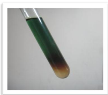
Figure.A. Libermann Burchard Test showing a brown ring for the presence of steroidal terpenoids in Centella asiatica L
